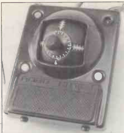
The Bit Stik controller includes three buttons as well as the joystick; a power-on light occupies the top-right position.
